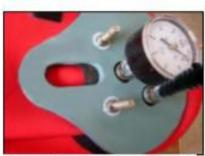
1. Provide air into the suit, through the foot pump, to a pressure of 0,7 to 1,4Kpa (0.1 to 0,2psi) [acc. MSC/Circ.1114.] Maintain pressure to those limits for the air-test. (It is normal that some bubbles appear at the zipper slides and at the zipper toothed part in the face fixture).
