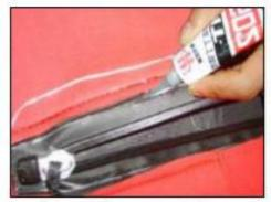
2. Apply a gentle amount of glue on the marked leaking areas. Let it dry for 8-10 minutes. Then apply once again, a glue layer on the immersion suit damaged area. Let it dry for 8 hours.
