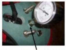
7. Insert the Pressure Gauge at the face fixture, by pressing down -at the same time- the joint at face fixture.
