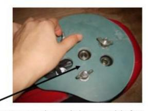
5. Install the o-ring gasket and tighten up the butterfly nut so as to eliminate leakage around the face seal.
