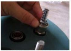
Install the Connector for the foot pump, by pressing down the proper joint, so as to insert it properly.
