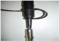
10. Adjust the multi-valve adaptor on the connector of face fixture.
