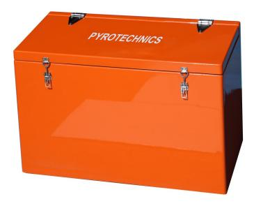
These chests are manufactured using Lloyds approved 3-4mm fire retardant GRP resins . This is backed up with an excellent IP rating of 56. It has both Lloyds and ABS approvals.
