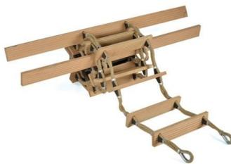
Hardwood (Beech Wood) Pilot Ladder, designed for safe and efficient pilot or crew transfer. Features include hardwood steps, rubber bottom steps for enhanced grip, 4-strand manila rope, and aluminium clamps. Wheelmark certified by Istituto Giordano, compliant with IMO Res. A.1045(27), ISO 799-1:2019, and SOLAS 74 Reg. V/23 & X/3, under Directive 2014/90/EU – Reg. (EU) 2023/1667, MED/4.49. Fully meets the latest IMO MSC 88 amendment standards.
