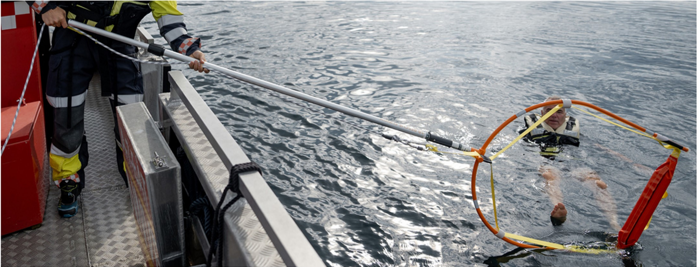
The SB Rescue Sling in action, using the 1m handle extension for a maximum usable length of 5.2m
