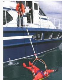
3. Pull on the line to release the harness from the frame and then push on the frame to tighten the harness around the casualty
