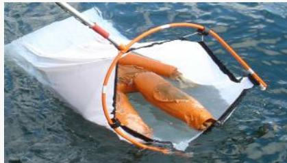
2. Pull on the line to release the bag from the frame
