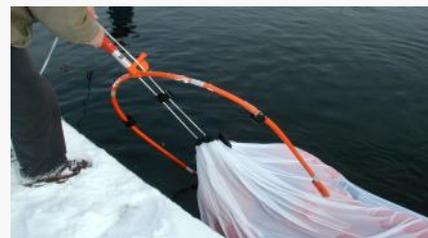
3. Push on the frame to tighten the drawcord and close the mouth of the bag, remove the frame and put to one side
