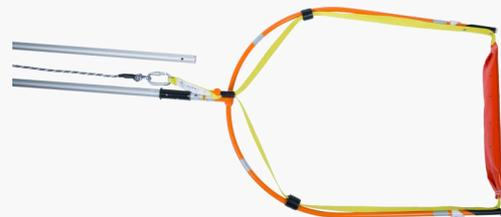
6. Fit the handle and telescopic extension, ensuring that all locating lugs are fully engaged. To adjust the telescopic extension unscrew the black plastic collar, slide the inner pole to the required position and then re-tighten the collar
