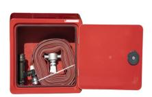
The JB85.360H fire hose cabinet is designed for harsh environments and offshore use. It features a durable 316 stainless steel hose pin and Lloyds-approved composites with UV-resistant gelcoats. The cabinet has an IP rating of 56, Lloyds and ABS approvals, and a lightweight but rigid design. The door has left or right hinging, an EPDM seal, and a graphite nylon rotary handle with Biomaster(R) technology. An anti-tamper seal can be added for security. This model replaces the JB16.360HR.
