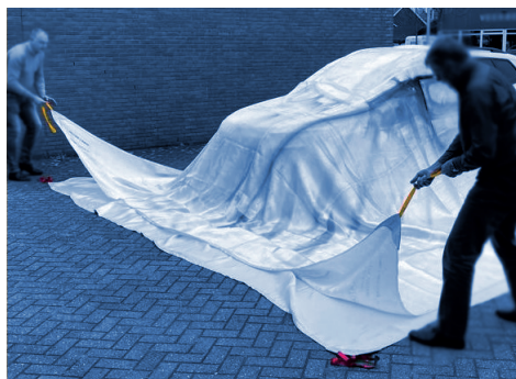
Start second part covering by using the red or yellow loops
