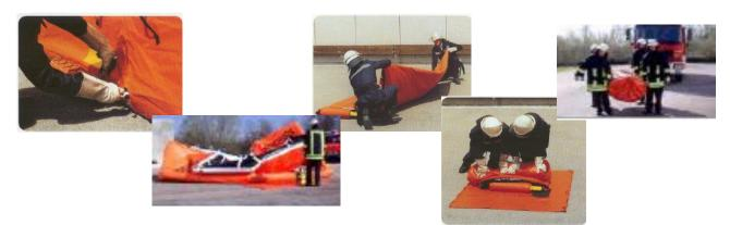
Open the deflate valves. Fold and roll the unit back into its valise.
