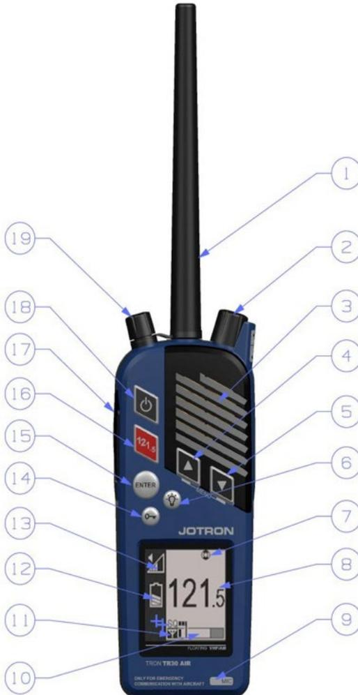
Figure 3 Tron TR30 AIR components
