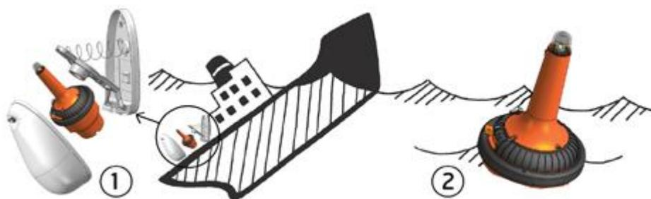
1. The Tron 40S MkII will automatically release from the bracket at a depth of 2-4 meters (6-13 feet) and start to transmit when reaching the surface.
